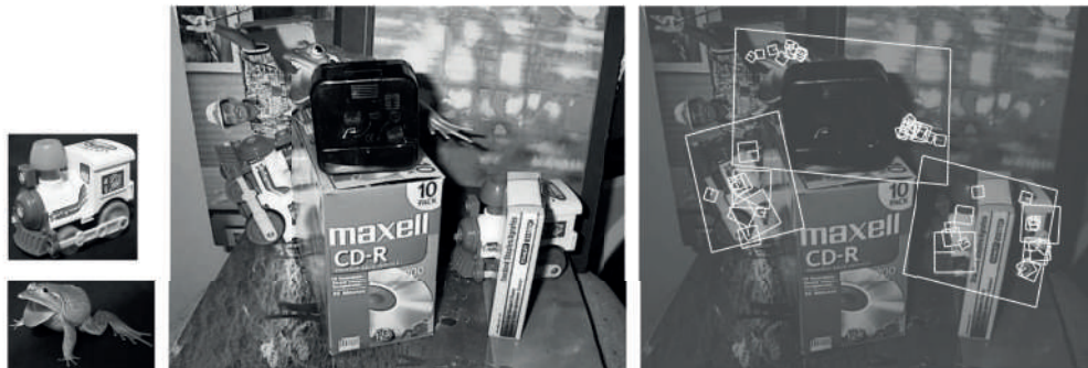
Figure 3.1: This figure, obtained from the original SIFT paper [89], illustrates how applying this algorithm could enable object detection from a complex scene by focusing on the most salient aspects of signals, the images on the left.
