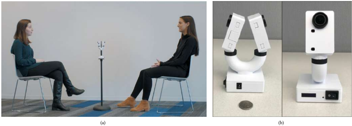
Figure 1: Experimental setup and data collection hardware. In (a), the participant and confederate are having a conversation with the “BioSensor” camera (a slightly older model shown here) placed between them. In (b), the current model of “BioSensor” used for data collection is shown.
