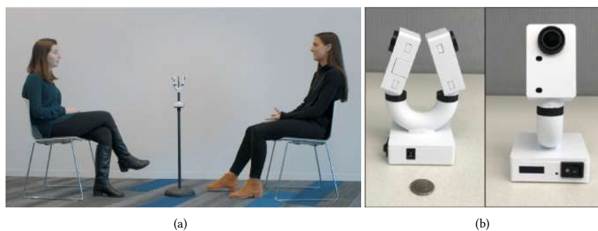
Fig. 1. Experimental setup and data collection hardware. In (a), the participant and confederate are having a conversation with the “BioSensor” camera placed between them. In (b), the current model of the “BioSensor.”
