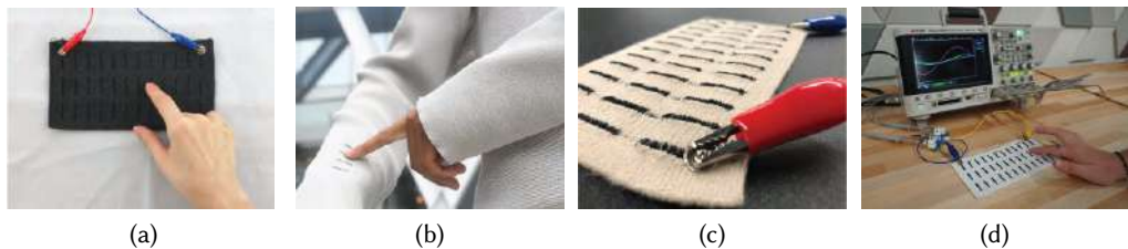
Fig. 1. Examples of the knitted capacitive touch sensor created through our manufacturing process: (a) A planar knitted fabric touchpad made from polyester and carbon-suffused nylon connected to two electrodes. (b) The sensing circuit integrated into a knitted sleeve. (c) Button snap fasteners used to connect the textile to an external sensing controller. (d) Oscilloscope visualization of the voltage input and output from the fabric circuit.
