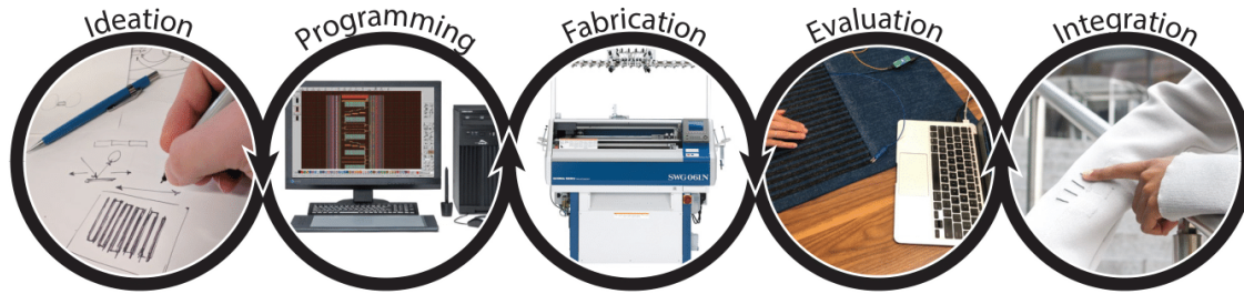
Figure 2: Knitted touch sensor design workflow: 1) Textile designers conceptualize sensor layouts while considering knitted circuit design guidelines. 2) The textile layouts are programmed using Knit Paint in the Shima Seiki SDS-ONE APEX3 software suite, and compiled for the desired weft knitting machine. 3) The compiled programs are transferred to the configured knitting machine for assembly. 4) The completed sensors undergo testing and evaluation to assess performance. 5) The textile circuits are directly integrated into devices with no human intervention needed after assembly.
